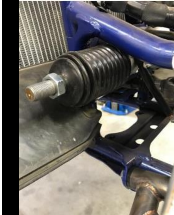
Figure 3: Steering boot installed over heim
