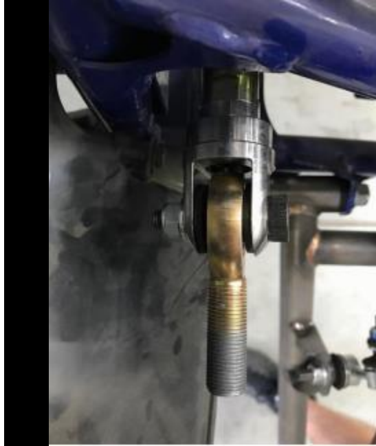
Figure 2: Install heim onto clevis.
