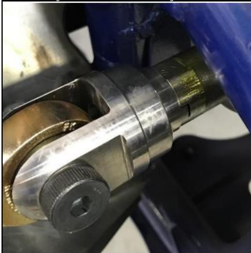
Figure 1: Install clevis onto steering box rack
