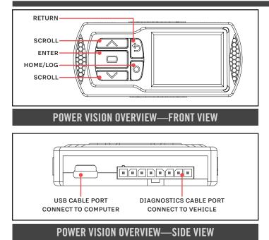
Thank you for purchasing the Power Vision from Dynojet Research. The Power Vision is the device to interface between your computer and vehicle ECU allowing you to tune your stock ECU to achieve optimal performance from your vehicle.
