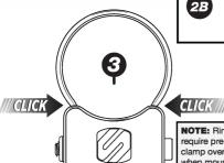
NOTE: Ring clamps 2" & over in size may require pre-stretching to help spread the clamp over the tube. (Use Protective film when mounting)
